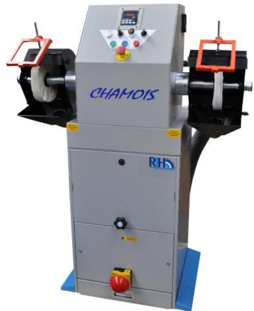
Extraction Mounted Powerfin Chamois shown with optional standard foot stop switch and optional lockable "E" stop
